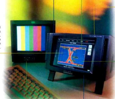
Long-term digital error logging can grab 400 complete errored frames for unattended burn-in and overnight testing.
